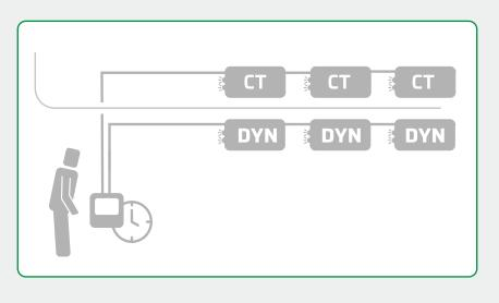
**CENTRALTEST** system makes use of 3 different communication technologies **CT, CTB** and **CTL** which determine the connection manner, wires types, addressing technique and maximum quantities of appliances. In one installation it is possible to use various communication technologies, combining them by means of a proper expander. All the technologies are based on EIA/TIA-485 and author's communication HELP protocol (Hybryd Emergency Lighting Protocol).
